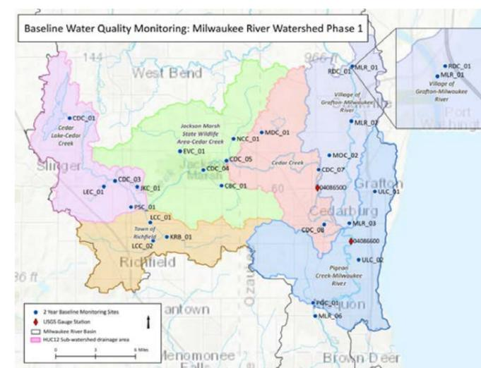
**Figure 1.** Locations (N=25) for collection of water quality data (TSS, TP, FC, *E. coli*, DO, pH, specific conductance, water temperature and turbidity) and continuous stage and discharge measurements in portions of the Milwaukee River Watershed.
